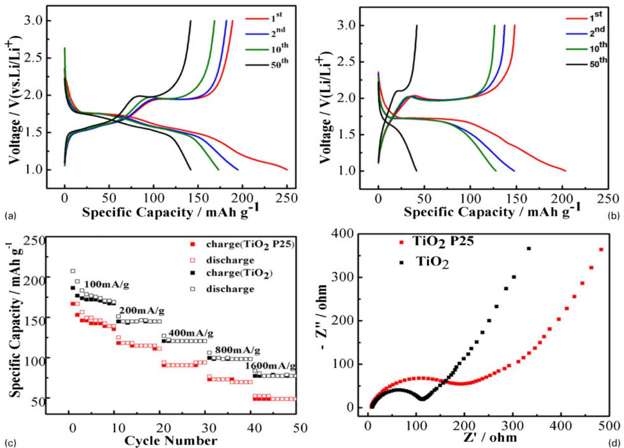
4 Charge/discharge curves for *a* hybrid TiO<sub>2</sub> nanowire array electrode and *b* P25 TiO<sub>2</sub> electrode at first, second, tenth and fiftieth cycles at current density of 100 Ma g<sup>-1</sup>; *c* charge/discharge capacities of hybrid TiO<sub>2</sub> nanowire array electrode and P25 TiO<sub>2</sub> electrode as function of cycle number at various current densities and *d* Nyquist plots of hybrid TiO<sub>2</sub> nanowire array electrode and P25 TiO<sub>2</sub> electrode
