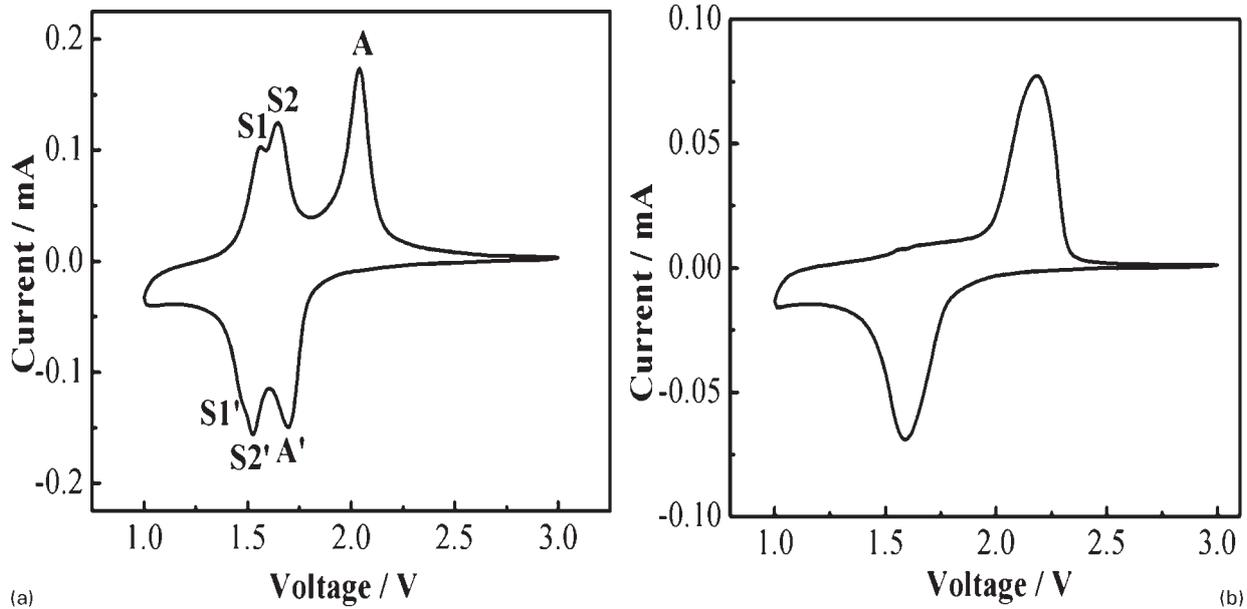
3 Cyclic voltammograms of *a* hybrid TiO<sub>2</sub> nanowire array electrode and *b* P25 TiO<sub>2</sub> electrode
