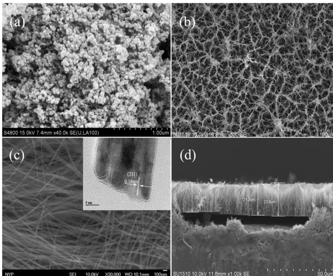
**2** *a* FESEM image of P25 TiO<sub>2</sub> nanoparticles, *b*, *c* FESEM images of hybrid TiO<sub>2</sub> nanowire arrays and *d* cross-section FESEM image of hybrid TiO<sub>2</sub> nanowire arrays (inset in *c* gives high resolution TEM of single TiO<sub>2</sub> nanowire)
