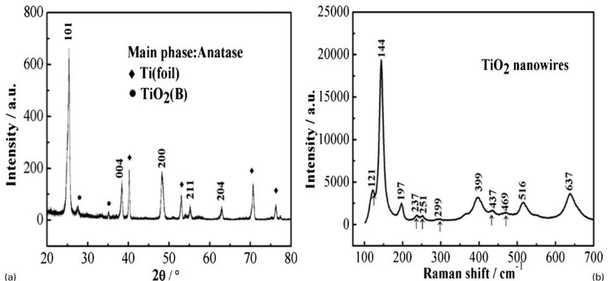
1 a XRD pattern of hybrid TiO<sub>2</sub> nanowire arrays and b Raman spectrum of hybrid TiO<sub>2</sub> nanowire arrays
